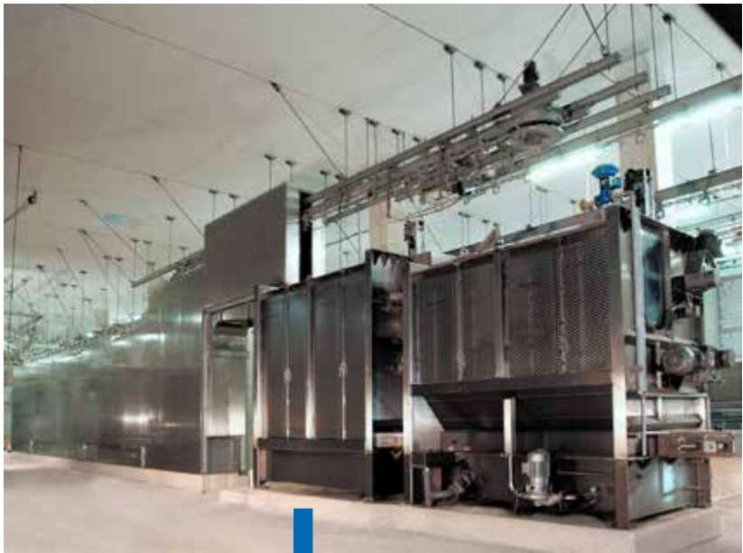
Self-supporting execution on a floor pedestal with housed transition into the continuous dehairing machine CDM
