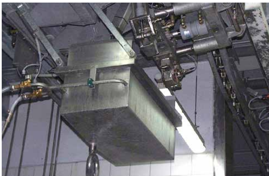
Cleaning and sterilisation unit for the holding tongs of the hook relief system of the roller dehydrator
