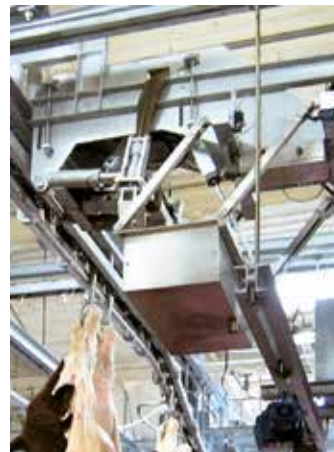
Hook release device with sterilization equipment
