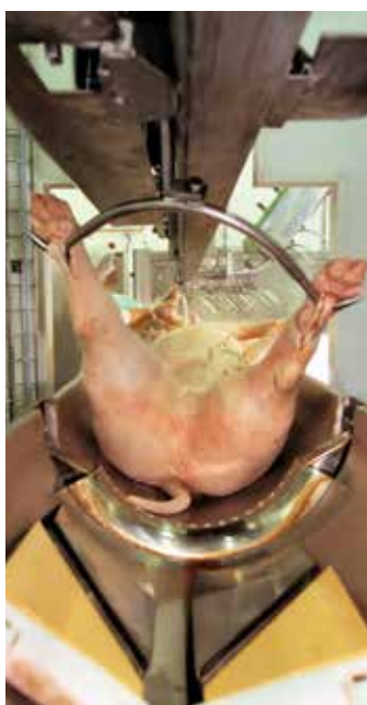
Conveying system combined with the automatic grading of pigs
