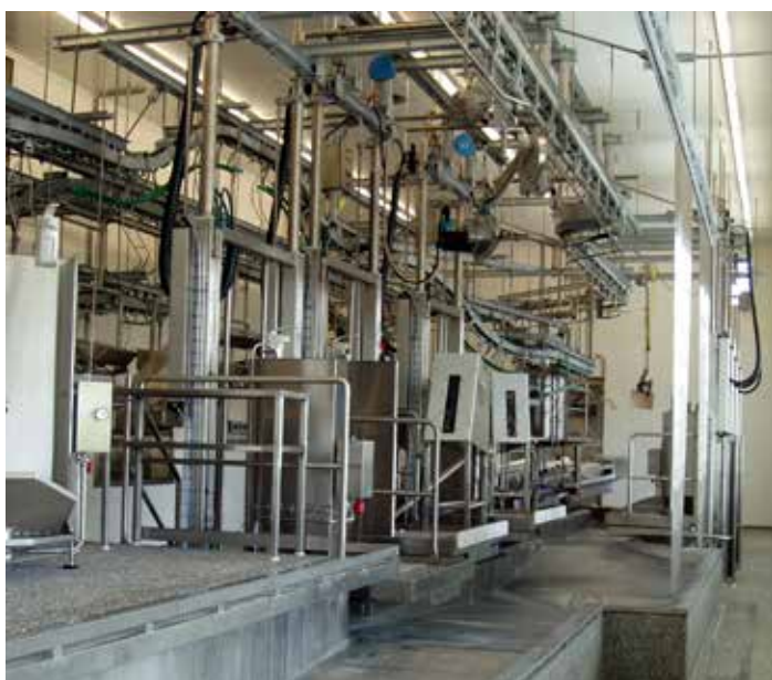
Lift and fixed platforms with sterilization stations for tools as well as cleaning equipment for the slaughtering operations
