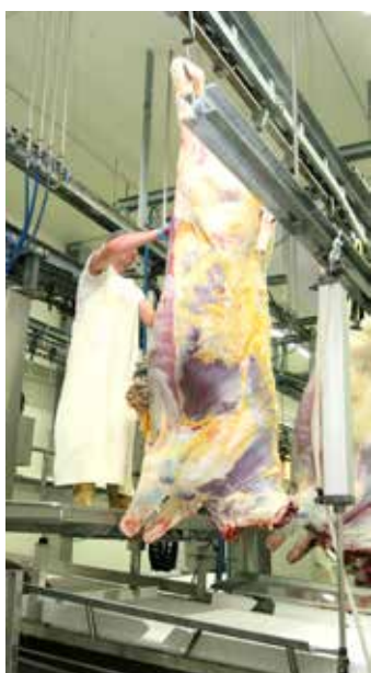
Ergonomic white offal removal and deposit directly into a tray, without any need for the operator to turn his body
