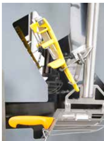
Automatic slaughtering knife cleaning and sterilization unit with ergonomic knife handling combines hygiene and ergonomics for best processing quality
