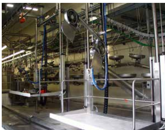
Horizontally and vertically moveable lifting platforms for handling of various carcass lengths and sizes
