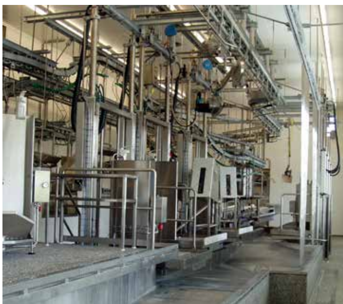
Lift and fixed platforms with sterilization stations for tools as well as cleaning equipment for the slaughtering operations
